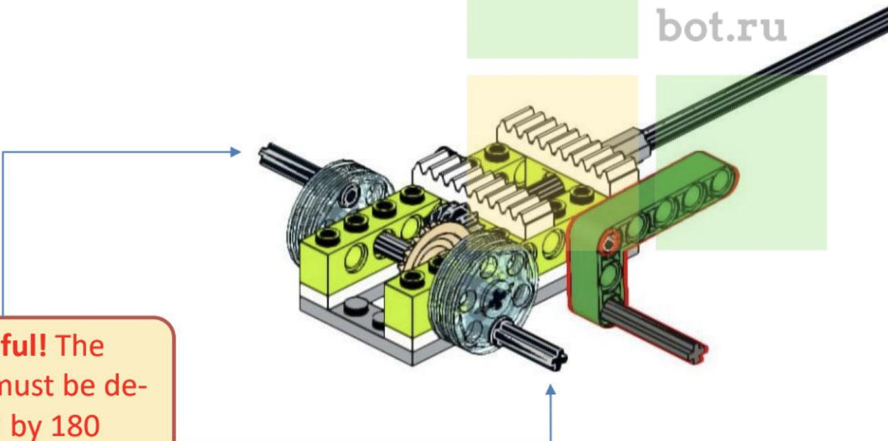
**Be careful!** The positions must be de-phased by 180 degrees to perform a correct walking motion!
